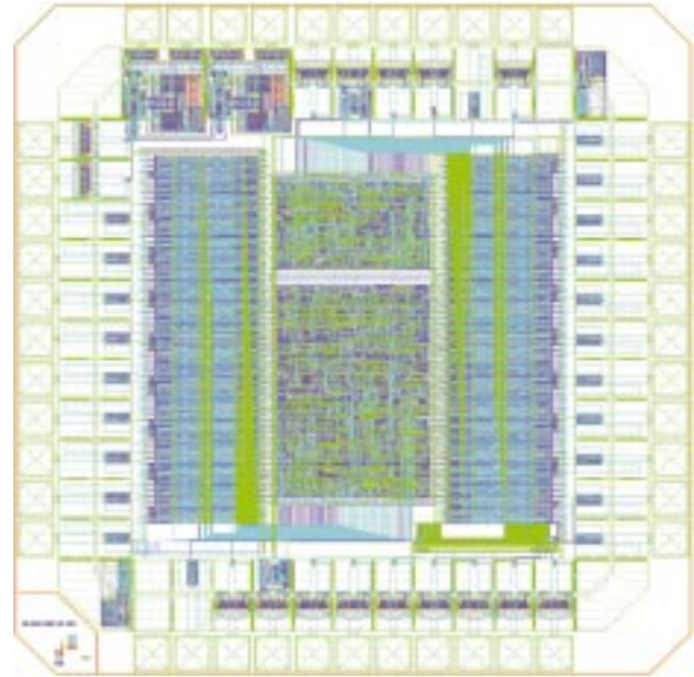
Figure 10: Layout of the BeetleSR 1.0 test chip. The two register blocks are located on the right and left hand side of the chip. The I 2 C interfaces are the blocks in the centre, the SEU robust one being the larger block.
