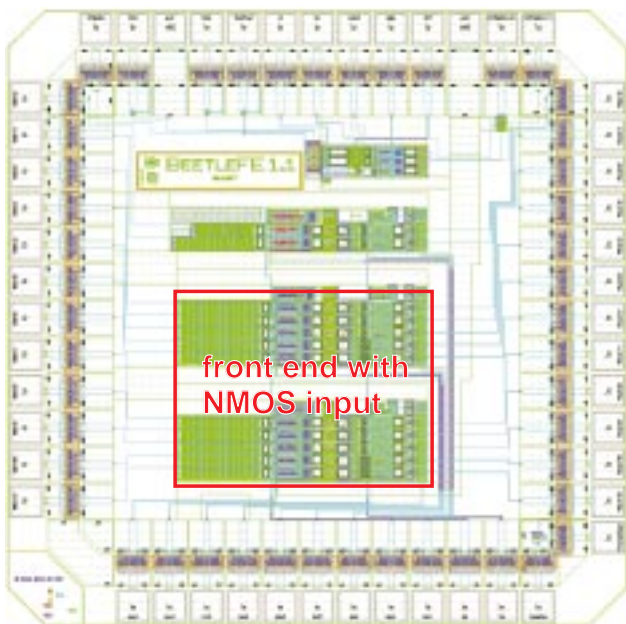
Figure 3: Layout of the BeetleFE 1.1 : The new front end channels are indicated
