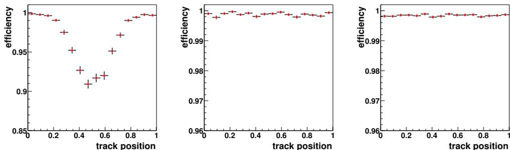
Figure 4: Efficiency versus track impact position for IT3 (left), Glast2000 (middle) and CMS (right).
