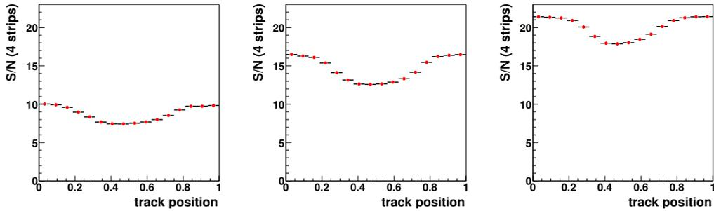
Figure 3: S/N versus track impact position in between readout strips for IT3 (left), Glast2000 (middle) and CMS-OB2 (right). On the abscissa, “0” indicates the center of the left strip and “1” the center of the right strip.
