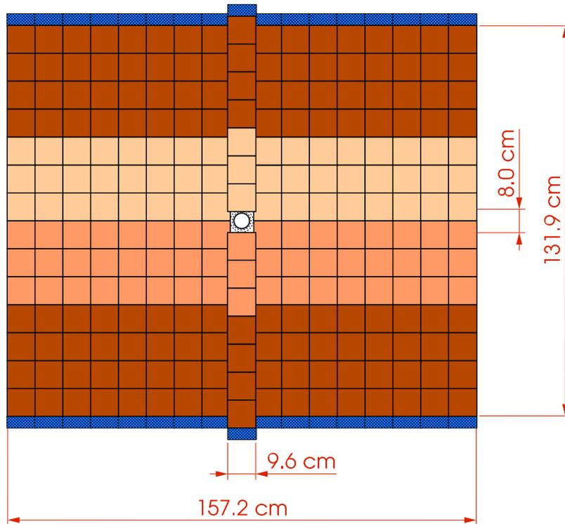
Figure 2: Layout of a TT detection layer. Readout sectors are indicated by different shading.
